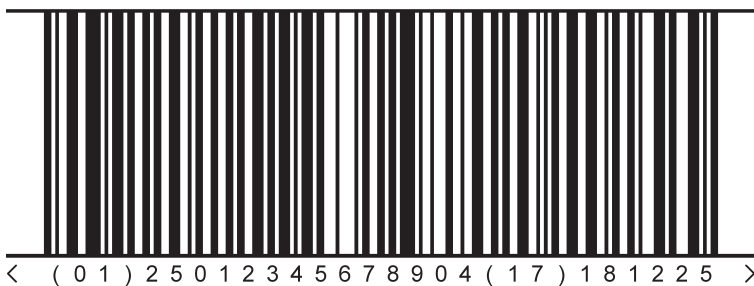
GS1-128 barcode with X-dimension of 0.50 mm
