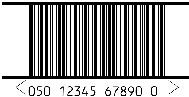
ITF-14 barcode with X-dimension of 0.495 mm
