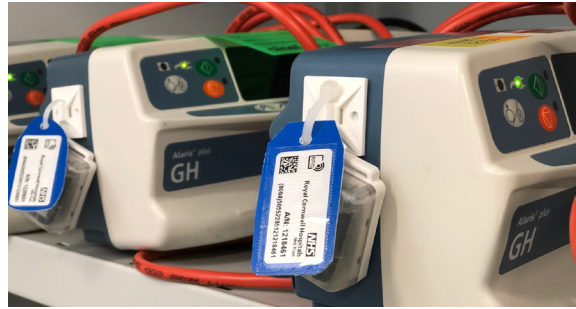
Medical device with a GS1 RFID asset label and a Wi-Fi tag
