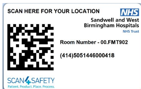
Sample of a physical location label – room level (using a GS1 DataMatrix 2D barcode)
