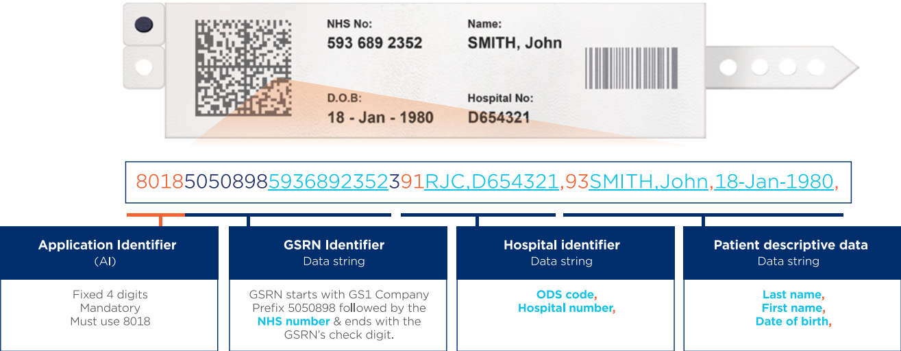
Figure 1: Example of a GS1-compliant patient wristband with encoded information
