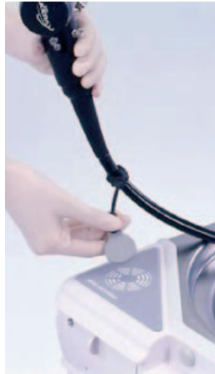
Fig. 4 IC tag attached to endoscope
