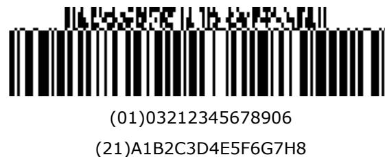
Figure 5.8.8-9. GS1-128 symbol with a four-column CC-A
