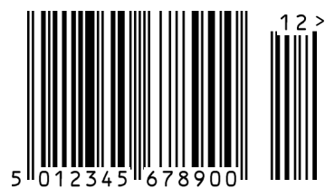
Figure 5.2.1.3.5.1-2. EAN-13 barcode with five-digit add-on symbol
