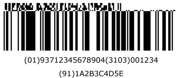
Figure 5.8.8-9. GS1-128 symbol with a four-column CC-A
