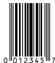
Figure 5.2.1.3.4-1. UPC-E barcode (encoding 001234000057 by zero-suppression)
