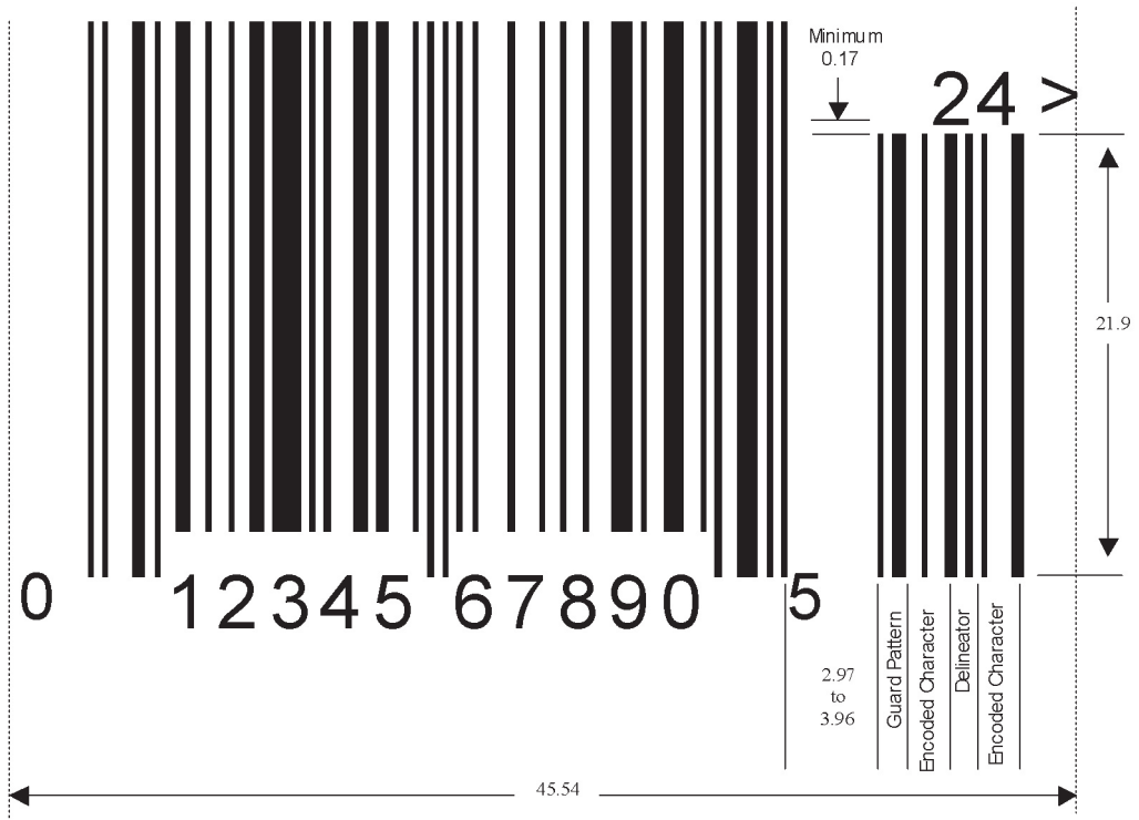
Figure 5.2.3.6-6. UPC-A barcode with five-digit add-on symbol
