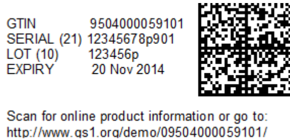
Figure 4.14.1-3. Combination of HRI with AIs, non-HRI text (GTIN and Expiry) and data titles
