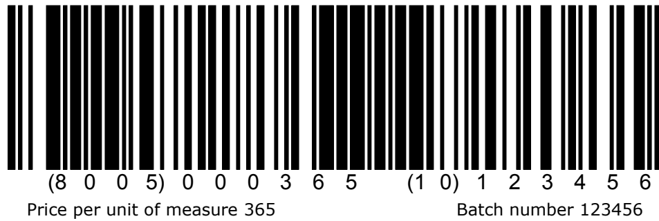
Figure 5.10.2.2-2. Data encoded in one concatenated GS1-128 symbol
