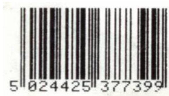
Figure 5.5.3.3.12-1. Symbol with edge determination problem
