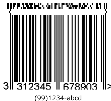
Figure 5.8.8-1. EAN-13 symbol with a four-column CC-A component
