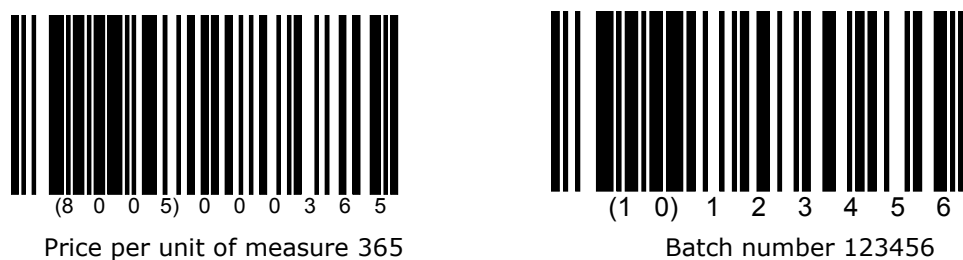
Figure 5.10.2.2-1. Data encoded in two GS1-128 symbols
