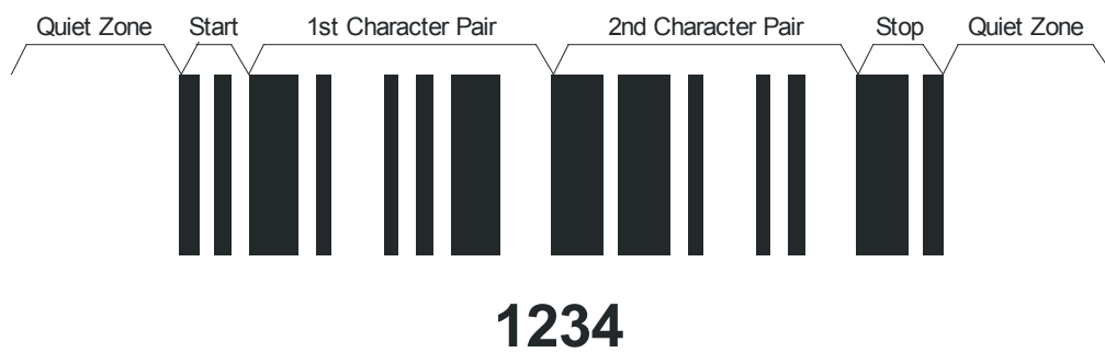
Figure 5.3.2.1.2-2. ITF-14 symbol inclusive of Quiet Zones
