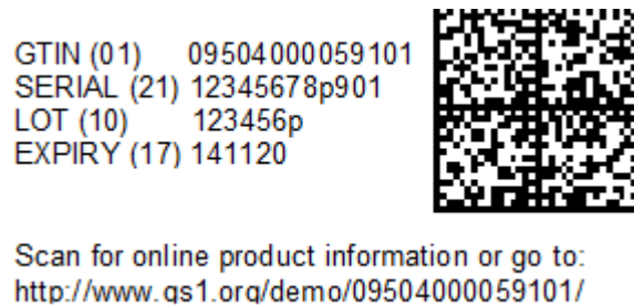
Figure 4.14.1-3. Combination of HRI with AIs, non-HRI text (GTIN and Expiry) and data titles
