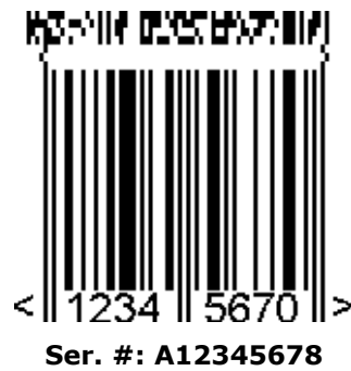
Figure 5.8.8-4. UPC-E symbol with a two-column CC-A
