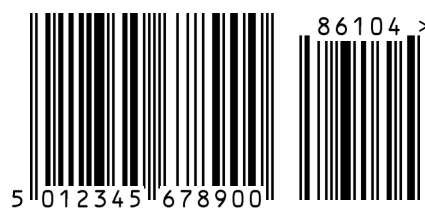
Figure 5.2.1.3.5.2-2. EAN-13 barcode with five-digit add-on symbol
