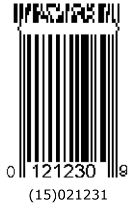
Figure 5.10.2.3-2. Example of mixed GS1 symbologies (GTIN encoded in UPC-E, Best before date in Composite)
