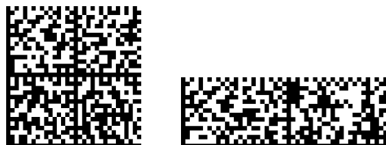
Figure 5.7.3.2-3. Segmented GS1 DataMatrix symbols: Square and rectangular formats (sizes of these GS1 DataMatrix symbols are larger than what would be used in a typical application so that typical alignment patterns can be easily seen.)
