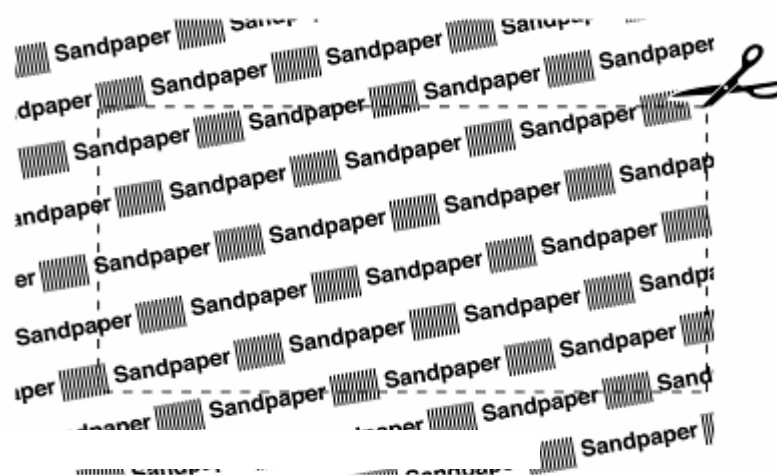
Figure 6.3.3.7-2. Barcode placement on random-wrapped item
