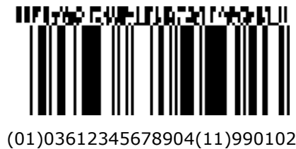
Figure 5.8.8-6. GS1 DataBar Stacked symbol with a two-column CC-A
