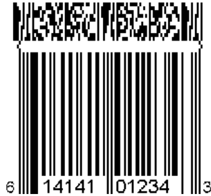
Figure 5.8.8-3. EAN-8 symbol with a three-column CC-A
