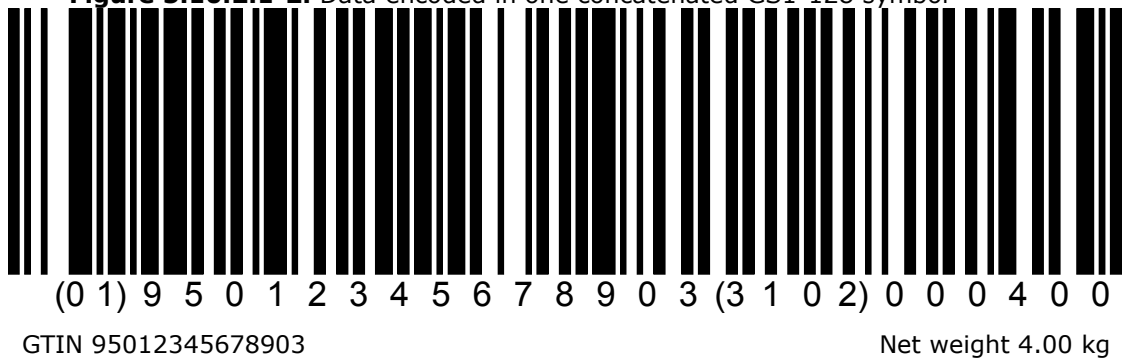
Figure 5.10.2.1-2. Data encoded in one concatenated GS1-128 symbol
