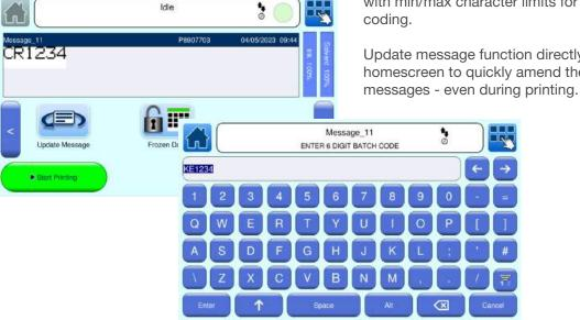
Messages can be stored in the printer for quick retrieval for fast product changeovers. You can also create, edit and store multiple line settings for quick changes between all your products or moving the printer between lines.
