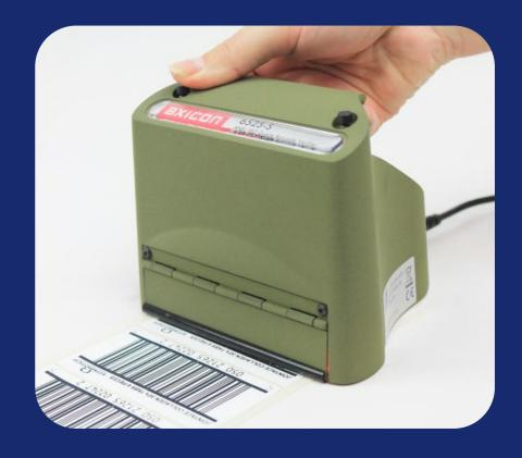
Results are immediately displayed on screen, and reports can be printed or e-mailed for remote diagnosis. Reports may be saved automatically to support ISO 9001 quality control procedures. Simple user-friendly calibration, and configuration of how results are displayed. This verifier is perfect for product manufacturers, label printers, printers and packagers, and pre-press studios. It is widely used by major retailers worldwide.
